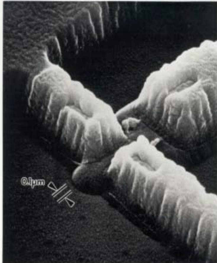
Ultra-short channel Si-MOSFET, IBM 0.5 μm wide, 0.1 μm channel
