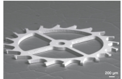
Scanning electron microscope picture of an anchor wheel coated with diamond like carbon containing ceramic SiC nanoclusters
